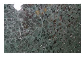
• The other reason that causes the glass breakage during heat soak test is unbalanced conditions during tempering. Heating or cooling the glass much over than enough may increase the stress level inside the glass. Stress level may be decided by counting the broken glass particles in a 5x5 cm area. If the amount of broken glass particles is quite much more than the limit
