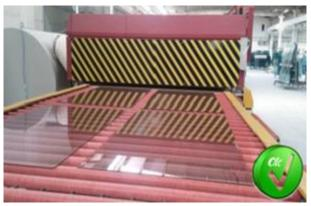
• Care must be taken that the upper set point of the temperature control unit do not exceed 685 °C. If it exceeds, roller print risk increase and some invisible defects like scratches, stains etc. at the coated surface, which formed at previous processes like cutting, deletion, edge grinding, drilling, washing etc., may become more visible after temper process.
