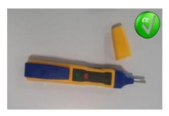
• In order to identify the edge deletion quality, coating detectors should be used.
