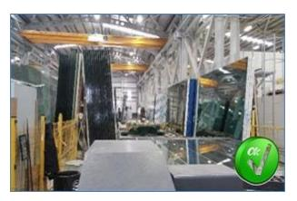
• The packaging material of glass packs (surrounding tape and silica gel) should not be removed until the cutting process. It is advised to consume all glass panes inside the pack once it is unsealed; if it is not possible, re-packing should be done very carefully.
