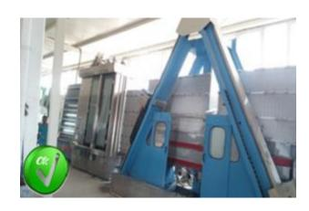
• For grinding process, an automatic horizontal (double edger, CNC etc.) or vertical grinding machines must be used. Glass must be transferred on conveyor system with coating side is not in contact with any conveyor elements.
