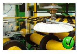
• Suction cups should be applied to the uncoated surface of coated glass. If contact with the coating is unavoidable, clean vacuum caps proper for coated glass should be used on suction cups. Şişecam Flat Glass suggest Eurotech MTC 2 brand of vacuum cap.
