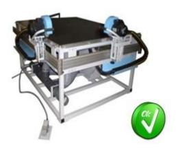
• At some projects, larger edge deleted areas (50 mm or wider) may be required especially at corner parts of the buildings. In similar cases, tempering problems like breakage, undulation etc. may be encountered. The reason of these problems are due to the fact that the edge deleted area of the glass is heated more rapidly than the area that is coated. Although generally it is not
