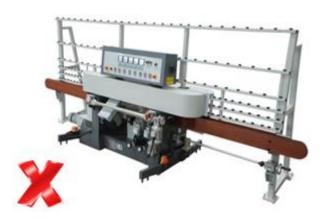
• For the horizontal edge grinding machines (double edger), top clamping belt must be smooth and non-textured in order not to damage the coated surface. Additionally, there must be a pulverize water nozzle and brush system to keep the upper belt wet and clean that located at entrance section.
